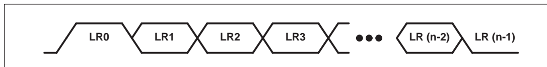
Each cell represents one clock sample time, and n is the number of bits in the request stream.
