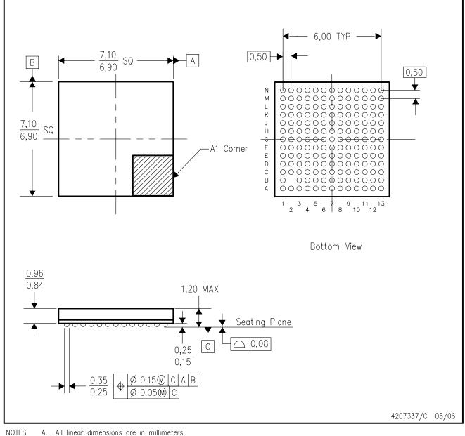
A. All linear dimensions are in millimeters.
