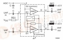
$V_{GG} = 5$  V: UHF AMP is on; VHF AMP is off  $V_{GG} = 0$  V: UHF AMP is off; VHF AMP is on (0 = shorted to Ground or open)
