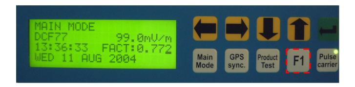
To activate the STORED SETTINGS MODE, the button F1 must be pushed.
