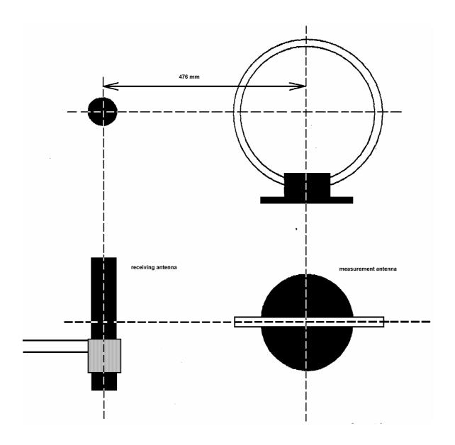
Between the shown generator idle motion voltage  $G_{\text{GEN}}\left[V_{\text{S}}\right]$  and the receiving field power under restriction of the above measurement set up following relation exists.
