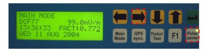
To activate the HARDWARE CALIBRATION MODE of the TSG400, the buttons and PULSE/CARRIER must be pushed >2 seconds.
