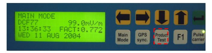
To activate the PRODUCTION TEST MODE, the button PRODUCT TEST button must be pushed.
