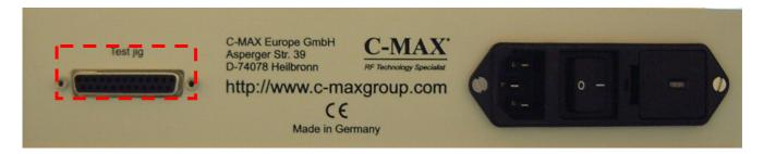
The test jig must be connected to the SUB25 parallel connector at the back side of the TSG400.
