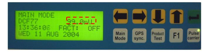
The cursor can be positioned onto the three possible digits for value adjustment or point onto the corresponding unit of the output voltage/field strength. The desired value can be adjusted with the and buttons. If the cursor is positioned onto the unit, the unit for output voltage /field strength can be increased or decreased with the and buttons.
