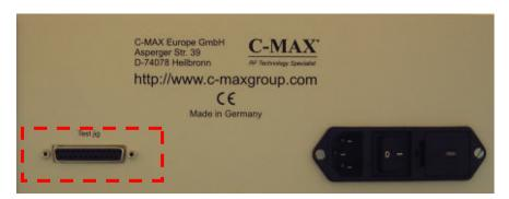
The test jig must be connected to the SUB25 parallel connector at the back side of the TSG800.
