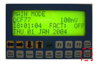
To activate the PRODUCTION TEST MODE, the button PRODUCT TEST button must be pushed.
