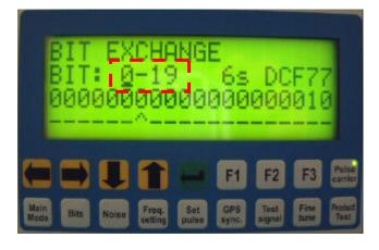
2. After selecting the bit range, move cursor with button to bit setting level and adjust bits with and buttons to the desired value.
