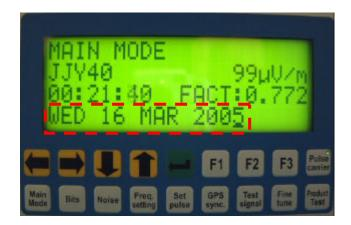
The cursor may be positioned onto date, month and year. The chosen value can be increased or decreased with the buttons and . If a date has been chosen which is larger than the length of the displayed month, the date is automatically adjusted to the largest allowed value. The adjustment of the year is possible from 2000 up to 2099. The day-of-the-week is calculated automatically.
