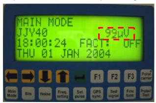
The cursor can be positioned onto the three possible digits for value adjustment or point onto the corresponding unit of the output voltage/field strength. The desired value can be adjusted with the and buttons. If the cursor is positioned onto the unit, the unit for output voltage /field strength can be increased or decreased with the and buttons.
