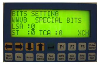
Furthermore, the anoncement bit for the leap second can be switched (LSA L= Leap Second Announcement)
