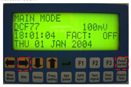
To activate the HARDWARE CALIBRATION MODE of the TSG800, the buttons and PULSE/CARRIER must be pushed >2 seconds.
