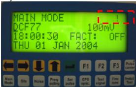
This option ( \binom{1}) is only available if values (other than noise, for noise adjustment, refer to 3.2.7)) have been adjusted, that are deviating from the standard values. By positioning the cursor below the icon \binom{1} and pressing the ENTER key, the standard values can be adjusted, then, the \binom{1} option will disappear. Following standard values will be adjusted:
