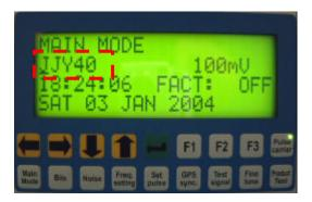
If the cursor is positioned onto any name of a time code transmitter, another transmitter can be chosen with the buttons and . Standard settings for the chosen transmitter will be valid at this time.
