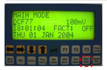
To activate the FINE TUNE MODE, the button FINE TUNE must be pushed.
