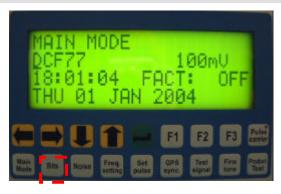
To activate the BIT SETTING MODE the corresponding signal must be chosen within the main mdoe and the button BITS must be pushed.
