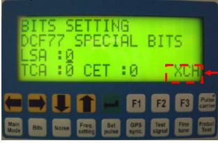
Also this mode offers a BIT EXCHANGE sub menu (XCH), where each single one of 60 bits of each protocol can be changed.
