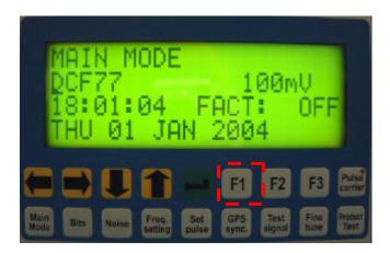
To activate the STORED SETTINGS MODE, the button F1 must be pushed.
