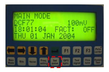
To activate the PULSE SETTING MODE, the button SET PULSE must be pushed.
