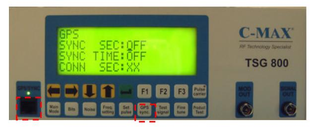
To start the GPS SYNC., push "GPS SYNC" button and connect the C-MAX "GPS100" unit by using the RJ45 GPS/SYNC. connector at the left side of the front panel.
