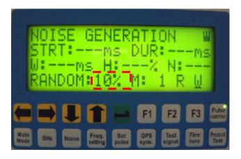
To activate RANDOM NOISE, the cursor must be placed at Random noise – OFF. By pushing the or button, a percentage for the random noise is selected. When Random is chosen, no other noise adjustment ist possible.
