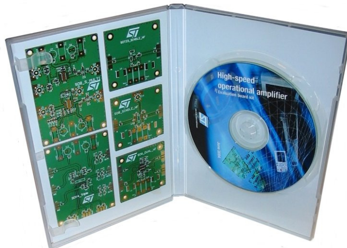
Figure 25: Evaluation kit for high-speed op-amps
