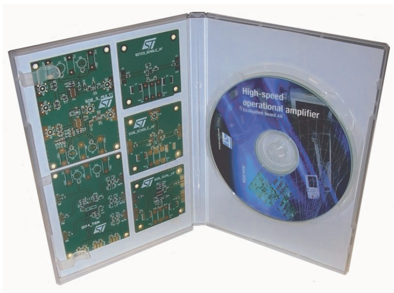
Figure 30. Evaluation kit for high-speed op-amps
