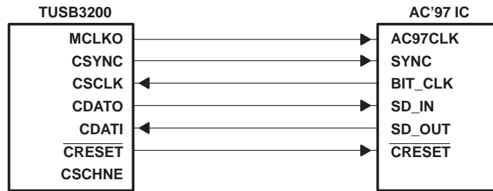
Figure 2–2. Connection of the TUSB3200 to an AC '97 CODEC
