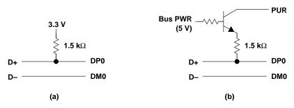
Figure 4–3. Upstream Connection (a) Non-Switching Power Mode (b) Switching Power Mode
