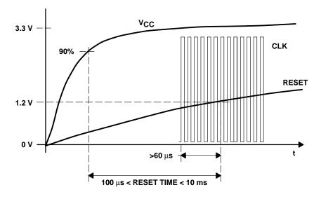
Figure 4–5. Reset Timing
