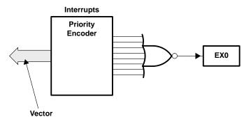
Figure 2–5. Internal Vector Interrupt (EX0)
