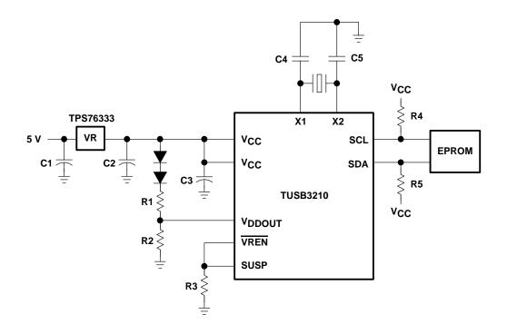
Figure 4–2. Partial Connection Bus Power Mode
