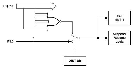
Figure 2–6. P2[7:0] Input Port Interrupt Generation
