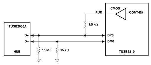
Figure 2–4. Pullup Resistor Connect/Disconnect Circuit
