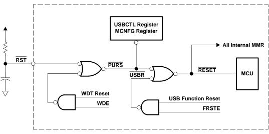
Figure 2–3. Reset Diagram
