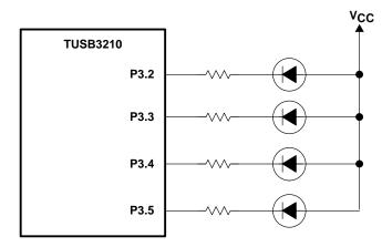
Figure 4–1. Example LED Connection
