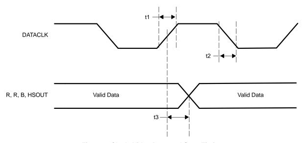
Figure 1. Clock, Video Data, and Sync Timing
