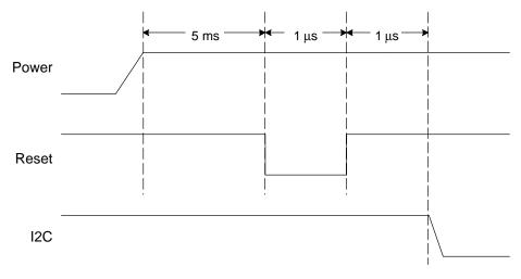
Figure 7. Reset Timing
