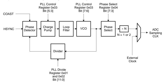
Figure 3. PLL Block Diagram
