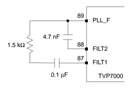
Figure 4. PLL Loop Filter
