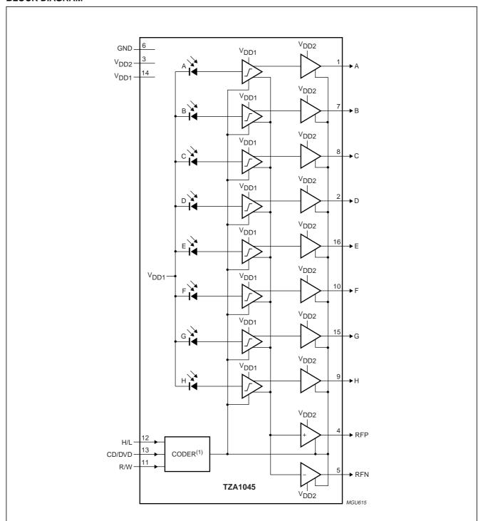
(1) The coder translates the three digital inputs into the appropriate gain level of each amplifier. The limiter is switched on only for CD-R writing for the segment outputs.
