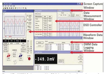
Figure 4 The U1600A Series comes with a PC Link application software that caters for data collection, storage and documentation needs via USB full-speed remote control from PC.
