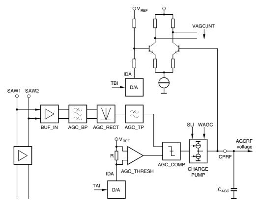
Figure 11. IFAGC Voltage-generation Block Circuit
