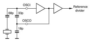
Figure 8. Oscillator Overdriven
