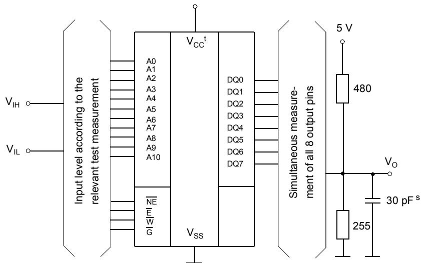
s: In measurement of  $t_{dis}$ -times and  $t_{en}$ -times the capacitance is 5 pF.
