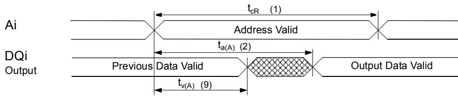
Read Cycle 2:  $\overline{G}$ ,  $\overline{E}$ -controlled (during Read cycle:  $\overline{W} = \overline{NE} = V_{IH}$ )<sup>g</sup>
