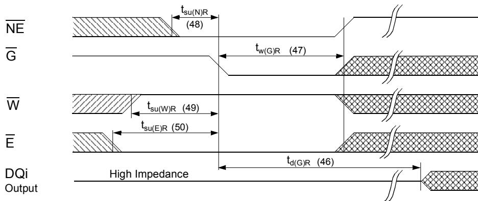
m: Measured with  $\overline{W}$  and  $\overline{NE}$  both returned HIGH, and  $\overline{G}$  returned LOW. Note that STORE cycles are inhibited/aborted by  $V_{CC} < V_{SWITCH}$  (STORE inhibit).
