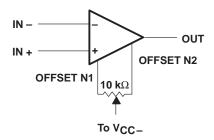
Figure 2. Input Offset Voltage Null Circuit
