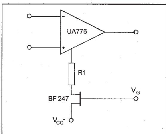
**OFFSET VOLTAGE NULL CIRCUIT**
