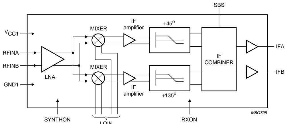
Fig.3 Block diagram, receive section.
