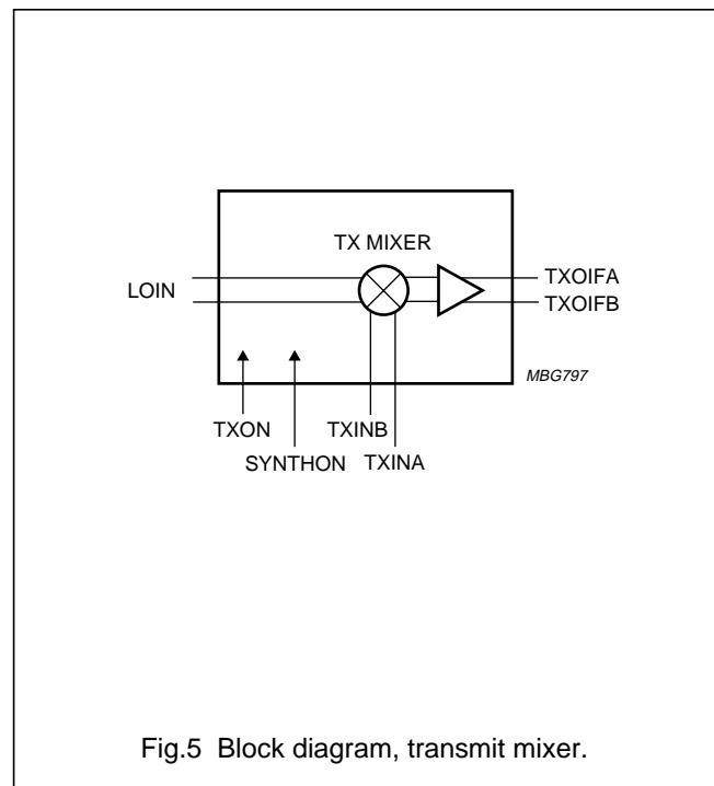
Fig.5 Block diagram, transmit mixer.
