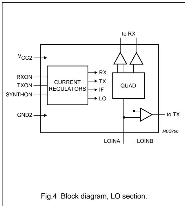
Fig.4 Block diagram, LO section.
