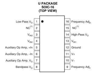
NOTE: (1) NC = no connection. For best performance connect all NC pins to ground to minimize inter-lead capacitance.
