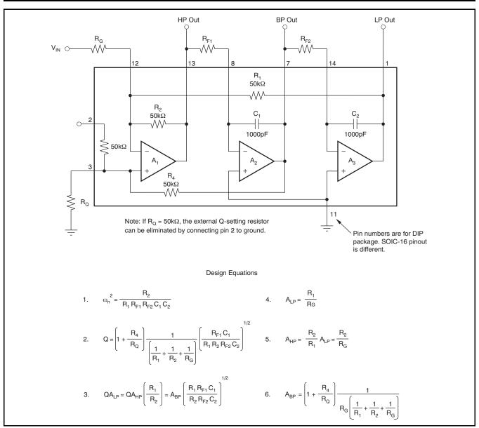
Figure 2. Inverting Pole-Pair
