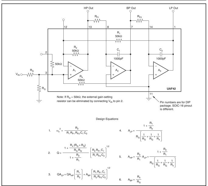
Figure 1. Noninverting Pole-Pair
