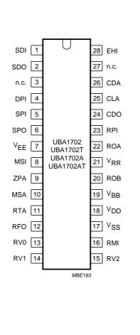
Fig.2 Pin configuration.
