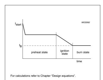
Fig.5 Operation in the preheat mode.
