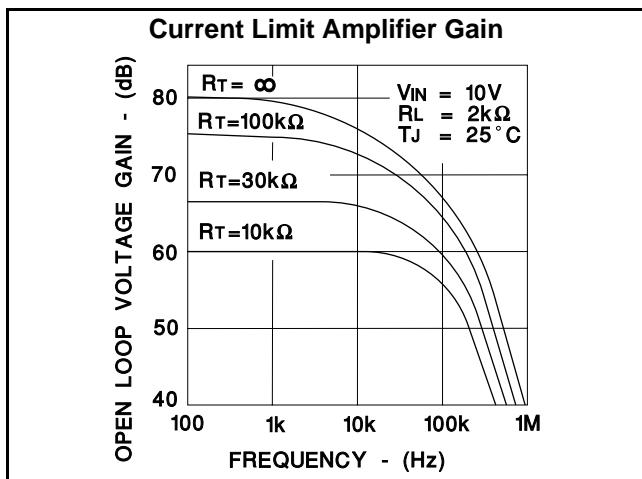
Note:  $R_T$  is connected from Offset Pin to Gnd. Values of  $R_T$  below 5.0k may cause Amplifier Cutoff at  $-55^\circ C$ .
