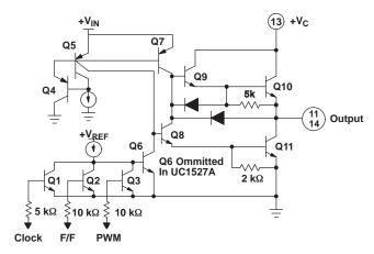
Figure 1. UC1525A Output Circuit (1/2 circuit shown)
