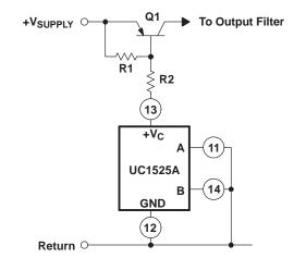
Figure 2. Grounded Driver Outputs For Single-Ended Supplies
