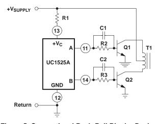
Figure 5. Conventional Push-Pull Bipolar Design
