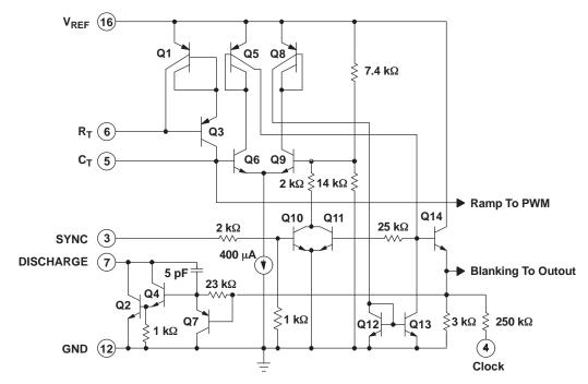
Figure 7. UC1525A Oscillator Schematic
