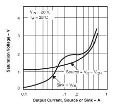
Figure 4. UC1525A Output Saturation Characteristics.
