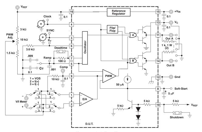
Figure 12. Lab Test Fixture
