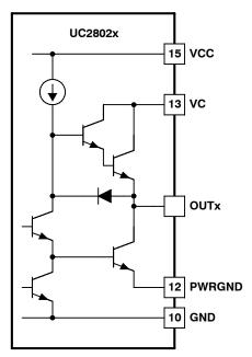
Figure 16. Simplified Schematic
