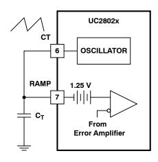
Figure 5. Voltage Mode Control
