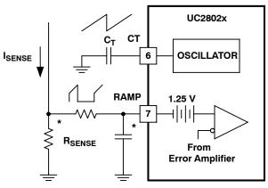
\* A small filter may be required to supress switch noise.
