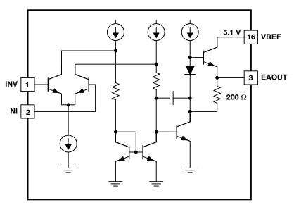
Figure 2. Simplified Error Amplifier Schematic
