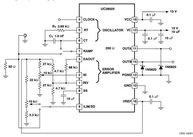
Figure 20. Laboratory Test Fixture
