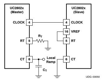
Figure 12. Synchronization of Two Units In Close Proximity
