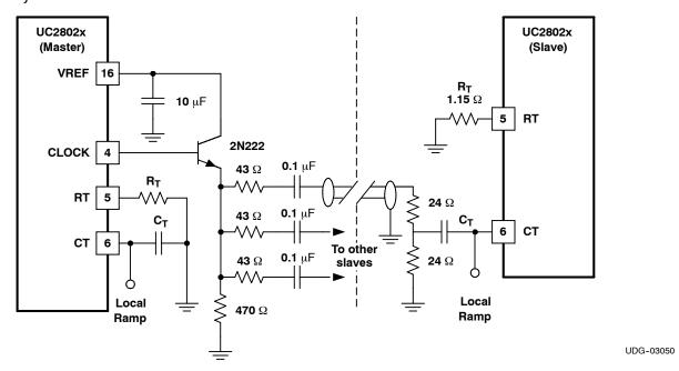
Figure 11. Generalized Synchronization
