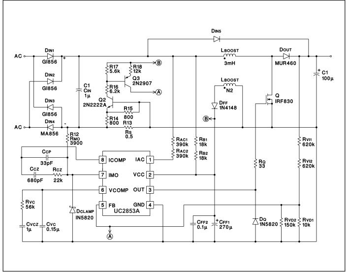
Note: the application circuit shown is a 100W, 63KHz design. Additional application information can be found in Application Note U–159 (TI literature Number SLUA080) and Design Note DN–78.
