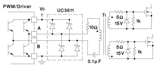
**Figure 4. Transformer Coupled Drive Circuits**
