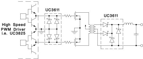
Figure 3. Clamp Diodes – PWMs and Drivers
