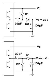
Figure 3. Charge pump circuits.
