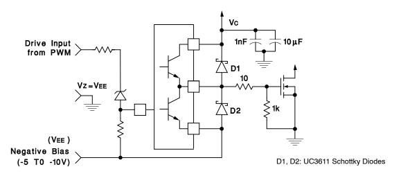
Figure 5. Power MOSFET drive circuit using negative bias voltage and level shifting to ground referenced PWM
