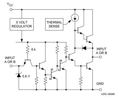
With inverting logic, these units feature complete TTL compatibility at the inputs with an output stage that can swing over 30 V. This design also includes thermal shutdown protection.
