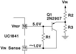
In this circuit, R1 is used in conjunction with CR (not shown) to establish a minimum ramp charging current such that the ramp voltage reaches 4.2V at the required maximum output pulse width.
