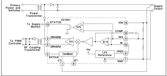
Figure 5. Feedback Coupled at Switching Frequency
