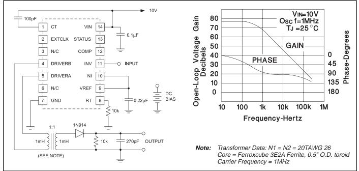
Figure 1. Transformer Coupled Open Loop Transfer Function
