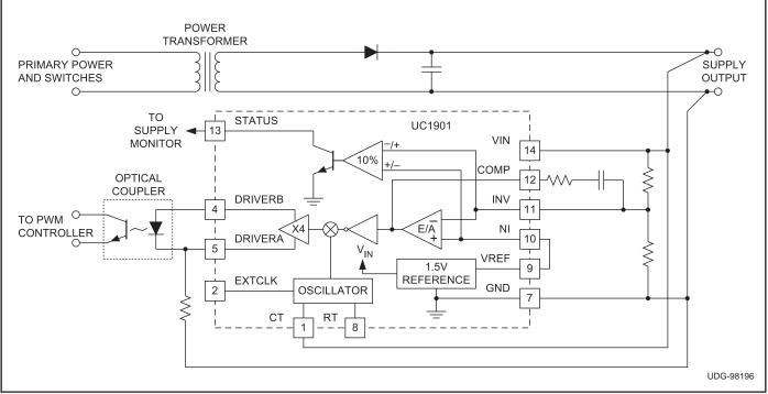
Figure 6. Optically Coupled DC Feedback
