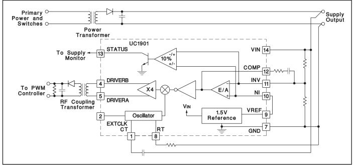
Figure 4. R.F. Transformer Coupled Feedback
