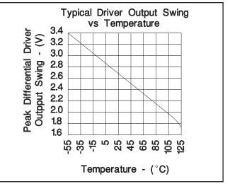
*Figure 3. Typical Driver Output Swing vs Temperature*
