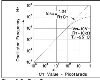
Figure 2. Oscillator Frequency
