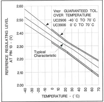
Internal reference temperature characteristic and tolerance.
