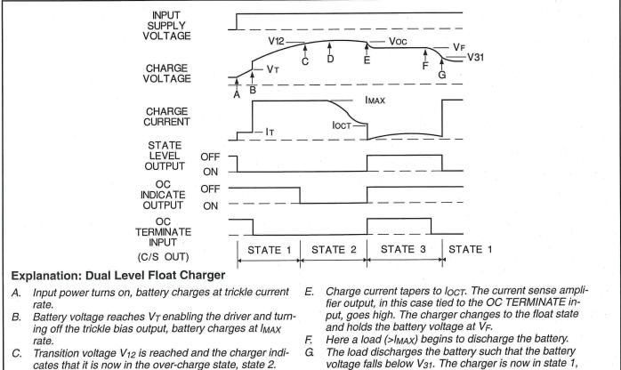
D. Battery voltage approaches the over-charge level V<sub>OC</sub> and the charge current begins to taper.
