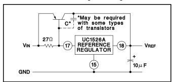
Figure 1. Extending Reference Output Current
