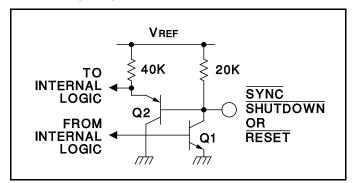
Figure 4. Digital Control Port Schematic
