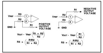
Figure 6. Error Amplifier Connections
