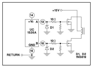
Figure 9. Driving N-Channel Power MOSFETs
