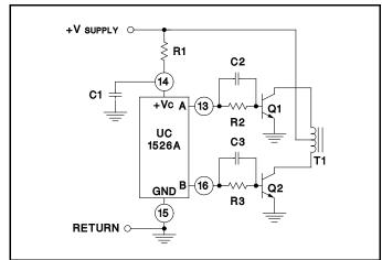
Figure 7 Push-Pull Configuration
