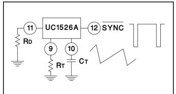
Figure 5. Oscillator Connections and Waveforms
