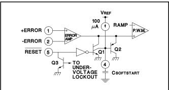
Figure 3. Soft-Start Circuit Schematic Digital Control Ports
