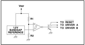
Figure 2. Under-Voltage Lockout Schematic Soft-Start Circuit
