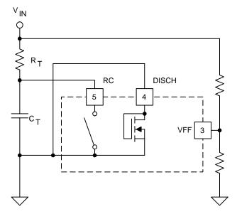
Figure 3. Ocsillator Without Clamp (MODE = 0)
