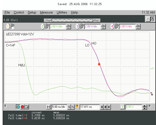
Figure 27. V_{LO} and V_{HO} Fall Time, 1-nF Load, 5-ns/Div
