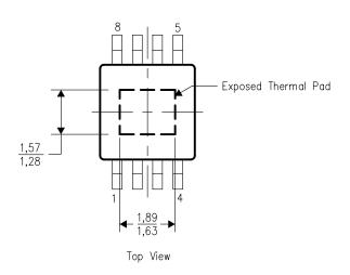
NOTE: All linear dimensions are in millimeters
