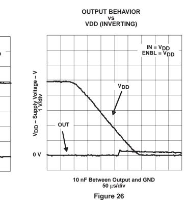
**OUTPUT BEHAVIOR** vs VDD (INVERTING)
