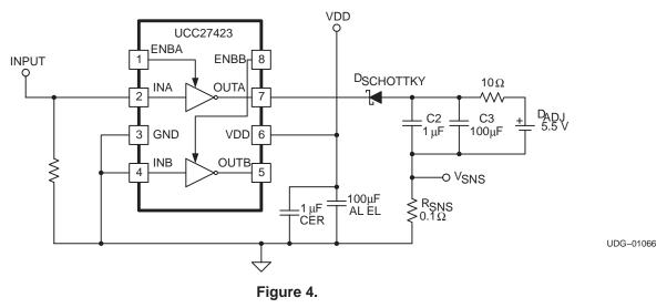
It should be noted that the current sink capability is slightly stronger than the current source capability at lower VDD. This is due to the differences in the structure of the bipolar-MOSFET power output section, where the current source is a P-channel MOSFET and the current sink has an N-channel MOSFET.
