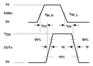
Figure 2. Switching Waveform for Enable to Output
