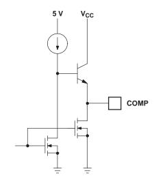
Figure 3. Error Amplifier Output Stage
