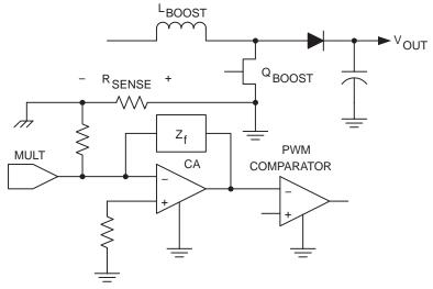
Figure 4. UCC3817 Current Amplifier Configuration
