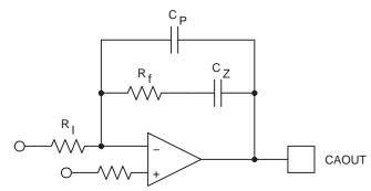
Figure 3. Current Loop Compensation
