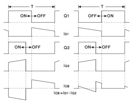
Figure 6. Timing Waveforms for Synchronization Scheme
