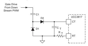
Figure 7. Synchronizing the UCC3817 to a Down-Stream Converter
