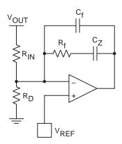
Figure 2. Voltage Amplifier Configuration
