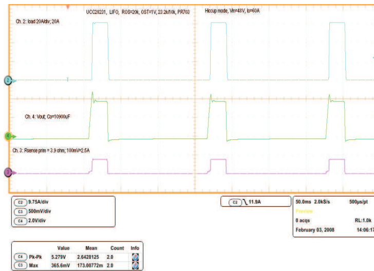
Figure 42. Cycle-by-Cycle Current Limit
