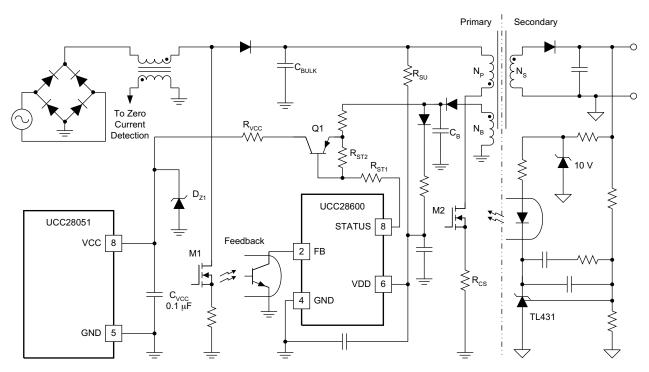
Figure 9. Using STATUS for PFC Shut-Down During Green Mode
