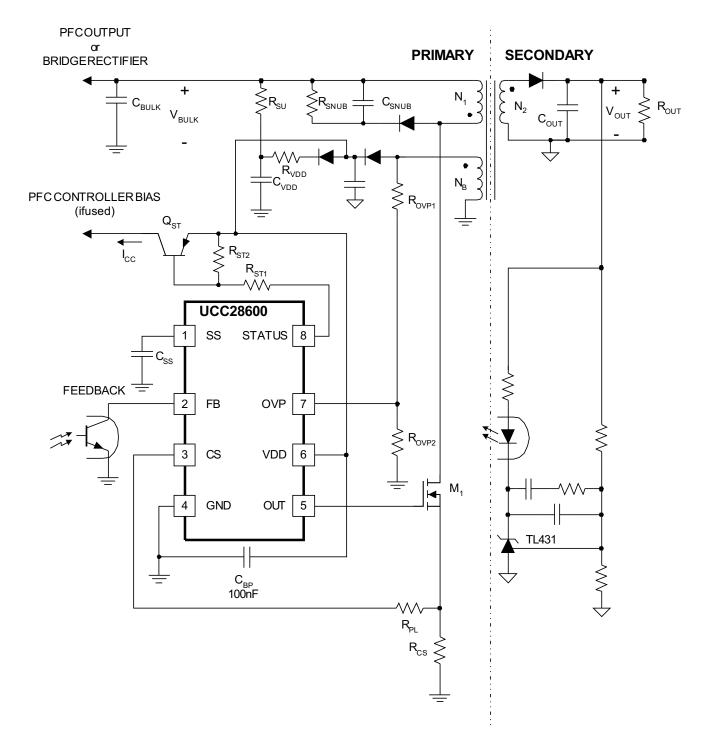
Figure 1. Pin Termination Schematic
