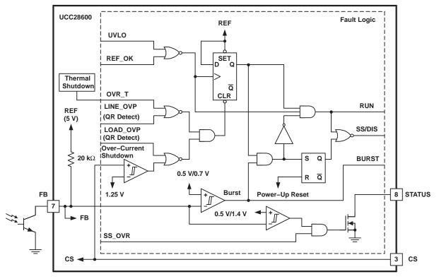
Figure 8. Fault Logic Details
