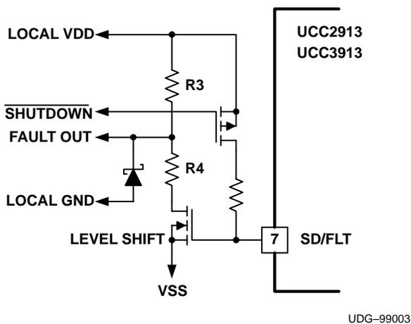
**Figure 4. Possible Level Shift Circuitry Interface**
