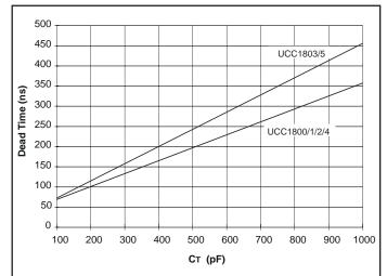
Figure 9. Dead time vs. C<sub>T</sub>, R<sub>T</sub> = 100k.
