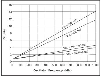
Figure 8. UCC1800 Icc vs. oscillator frequency.
