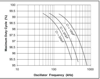
Figure 6. UCC1800/2/3 maximum duty cycle vs. oscillator frequency.
