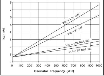
Figure 8. UCC1805 ICC vs. oscillator frequency.
