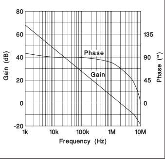
Figure 2. Error amplifier gain/phase response.
