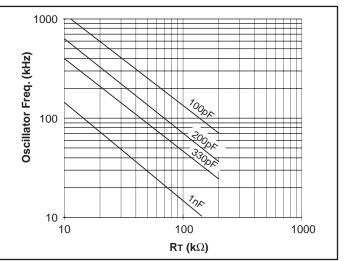
Figure 4. UCC1800/1/2/4 oscillator frequency vs. R<sub>T</sub> and CT.
