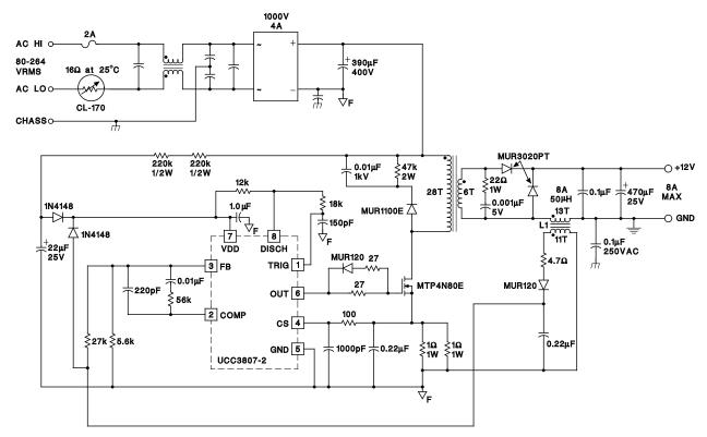
Figure 2. Typical Off-Line Application Using UCC3807-2
