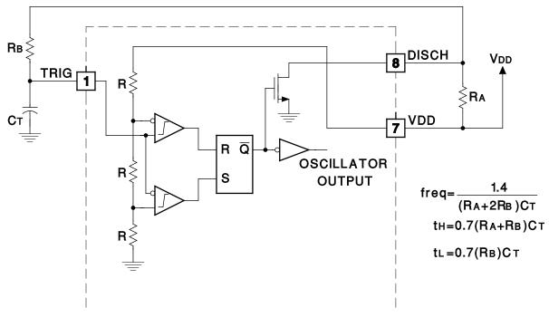
Figure 1. Oscillator Block Diagram
