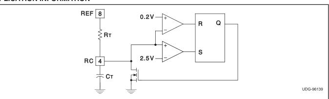
The UCC3813-0/-1/-2/-3/-4/-5 oscillator generates a sawtooth waveform on RC. The rise time is set by the time constant of  $R_T$  and  $C_T$ . The fall time is set by CT and an internal transistor on-resistance of approximately  $125\Omega$ . During the fall time, the output is off and the maximum duty cycle is reduced below 50% or 100% depending on the part number. Larger timing capacitors increase the discharge time and reduce the maximum duty cycle and frequency.
