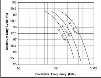
Figure 4. UCC3813-0/-2/-3 max. duty cycle vs. oscillator frequency.
