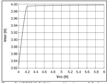
Figure 5. UCC3813-3/-5 V<sub>REF</sub> vs. V<sub>CC</sub>; I<sub>LOAD</sub> = 0.5mA.
