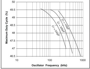
Figure 7. UCC3813-1/-4/-5 max. duty cycle vs. oscillator frequency.
