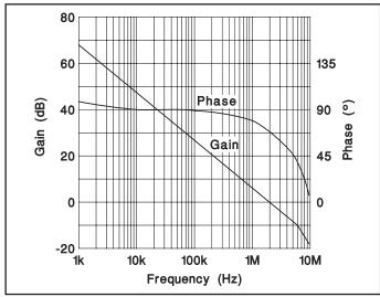
Figure 2. Error amplifier gain/phase response.
