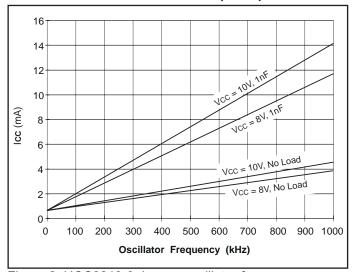
Figure 8. UCC3813-0 I<sub>CC</sub> vs. oscillator frequency.
