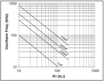
Figure 6. UCC3813-3/-5 oscillator frequency vs.  $R_T$  and  $C_T$ .
