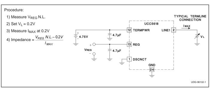
Figure 1. Termline Impedance Measurement Circuit
