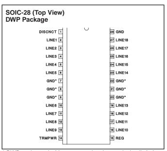
\* DWP package pin 28 serves as signal ground; pins 7, 8, 9, 20, 21, 22 serve as heatsink/ground.
