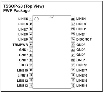
\* PWP package pin 23 serves as signal ground; pins 7, 8, 9, 20, 21, and 22 serve as heatsink ground.
