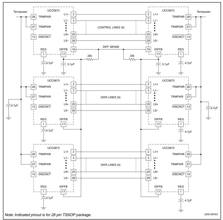
Figure 1. Application diagram.
