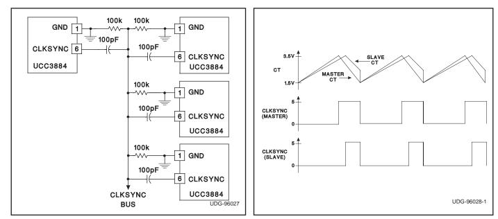
*Figure 2. Oscillator synchonization connection diagram.*
