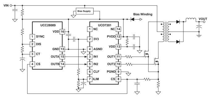
Figure 3. Intermediate Bus Converter
