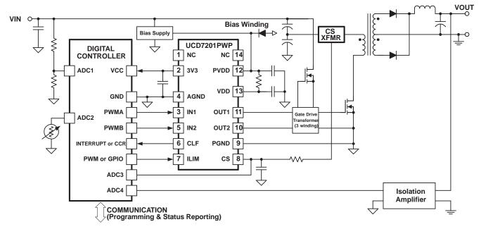
Figure 2. Half-Bridge Converter
