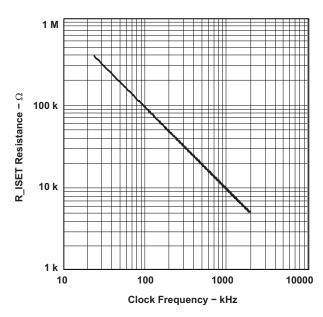
Figure 33. ISET Resistance vs Clock Frequency
