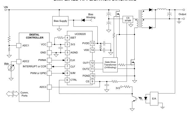
Figure 2. UCD8220 Typical Simplified Half-Bridge Converter Application Schematic
