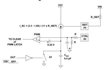
Figure 34. UCD8220 Configured in Voltage Mode Control with Voltage Feed Forward
