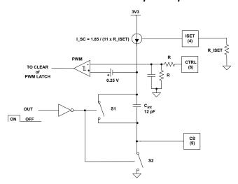
Figure 35. UCCD8220 Configured in Peak Current Control with Internal Slope Compensation
