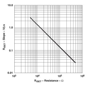
Figure 36. Slope vs RISET Resistance
