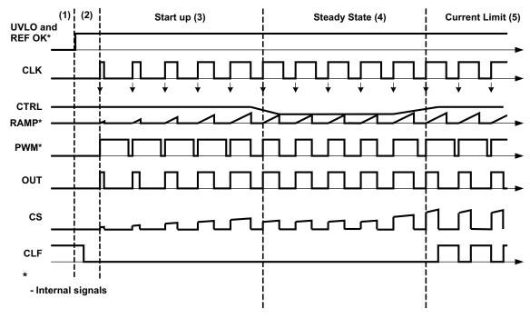
Figure 30. UCD8220 Timing and Circuit Operation Diagram
