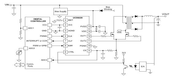
Figure 1. UCD8220 Typical Simplified Push-Pull Converter Application Schematic
