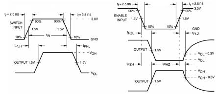
FIGURE 3. AC Waveforms
