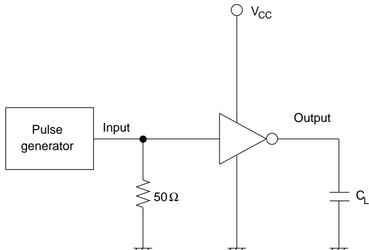
Note: Operating current test time, output is open.
