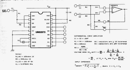
Figure 1. Single Ended Input Configuration
